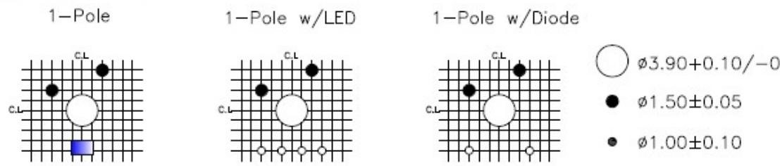
Keypad with Fixation Pins
